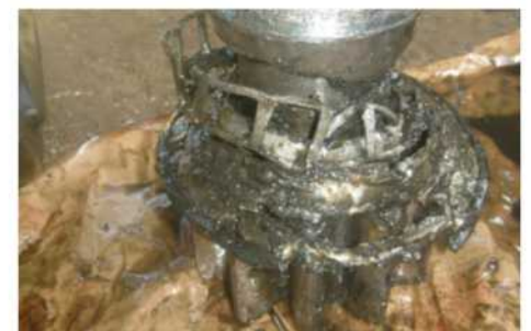
Bearing pinion patah
