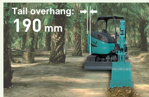
The tail overhang is 196 mm, which is within 10 % of the machine width complying with the Japanese definition of SR (Short Radius).
