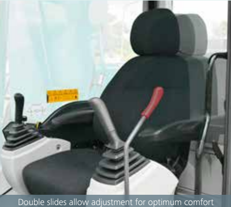
Double slides allow adjustment for optimum comfort
