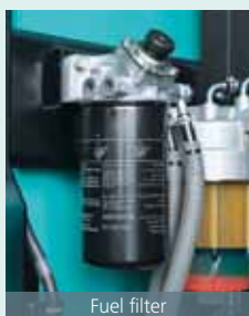
Fuel filter with built-in water-separator
