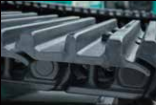
Reinforced HD shoes of thick steel plate to master rough, stony ground.
