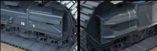
Reinforced guide frame prevents deformation caused by impact or encroaching of loose stones.
