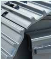
Increased shoe plate thickness
