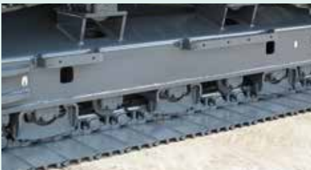
Track guides installed in three places
