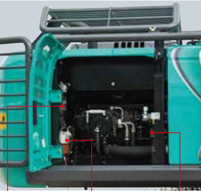
Fuel filter Fuel filter with built-in water-separator Engine oil filter
