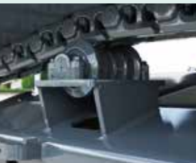
Double-Support outer flange upper rollers
