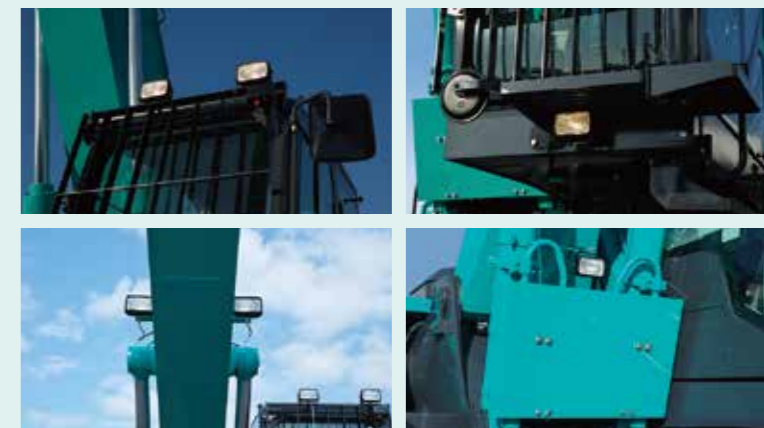
•Top left: 2 cab lights •Top right: Cab foot light •Bottom left: 2 boom lights •Bottom right: Boom cylinder light
