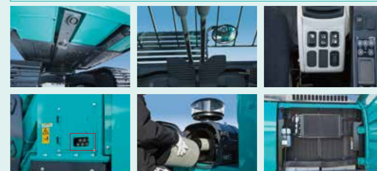
•Top left: Upper frame under cover •Top center: Cab foot mirror •Top right: Right console switches •Bottom left: Central lubrication (elevator cab) •Bottom center: Double-element air cleaner •Bottom right: Air conditioner condenser bug net
